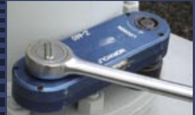
Z460 at work using standard ratchet wrench.
