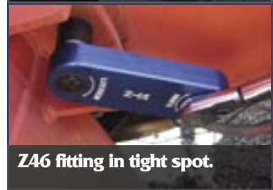
Z46 using the optional reaction arm.
